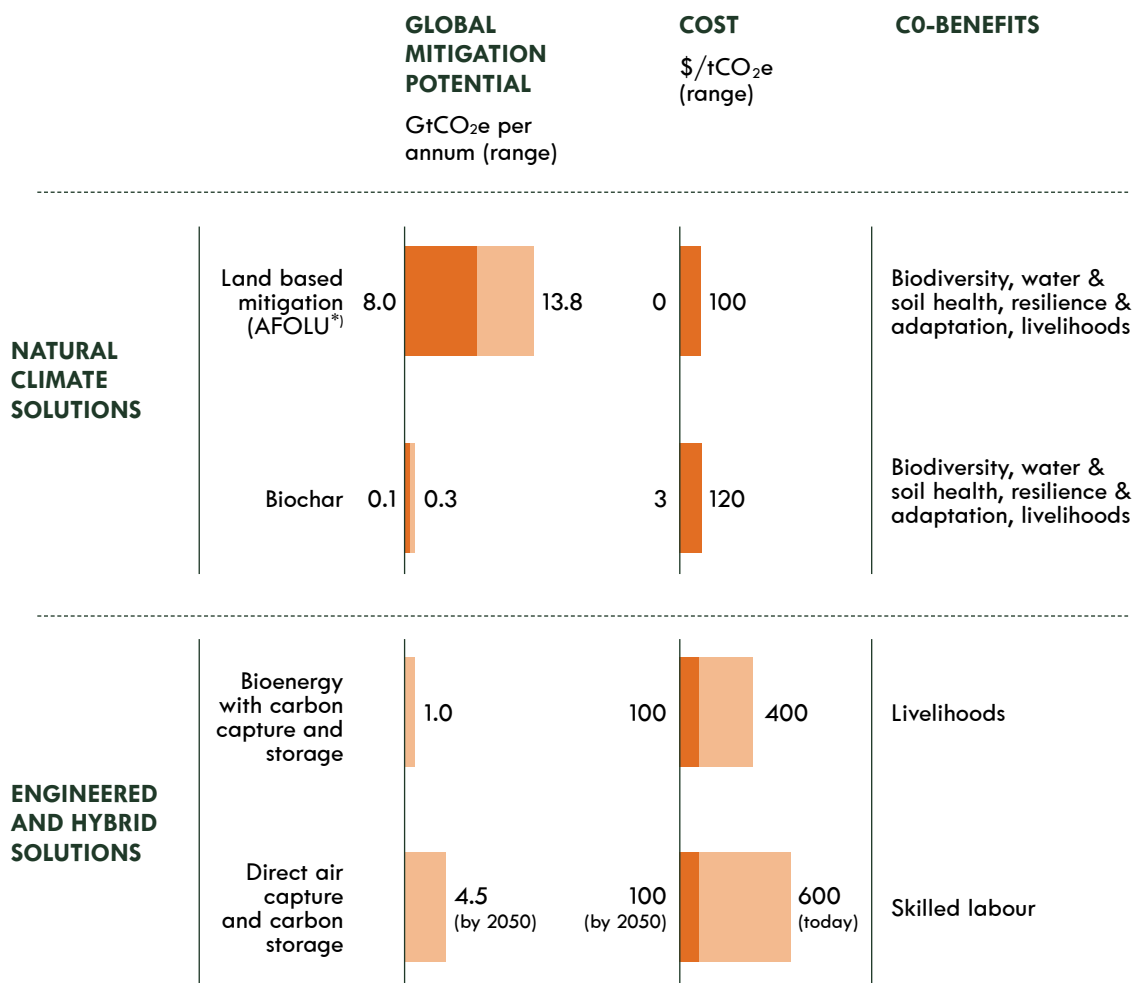
Figure 16: Natural climate solutions are more cost-effective than engineered solutions and offer more co-benefits
