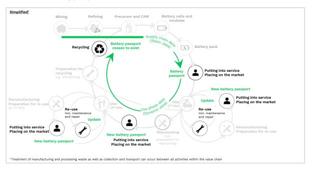
Figure 11: Battery life cycle and implications of battery handling operations on the data as well as start and end of the battery passport
