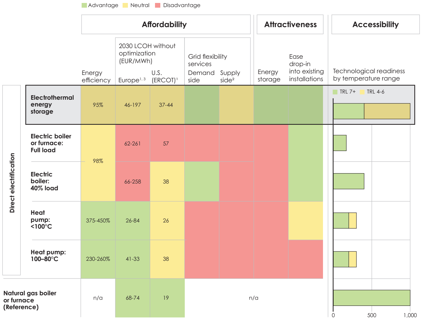
Figure 8 Key differences between ETES, heat pump and e-boiler technologies
